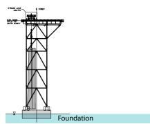
A strand jack gantry positioned atop the erection tower will lift the top of the tower segment, while a winch-assisted tipping cart will stabilize the segment and help move it down the rails. The tower section will pivot from a horizontal to a vertical position. The strand jack gantry will then lift the segment off the barge and into position onto the foundation.
